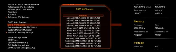
■ DDR5 XMP Booster: Predefined profiles for Micron, Hynix and Samsung IC manufacturers. Most of the times these profiles should work without a problem but it's not guaranteed. You can find your DRAM IC manufacturer at the right side of the bios screen and select one of the suitable profiles.
