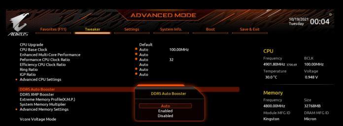
■ DDR5 Auto Booster: This option boosts the memory kit from its stock frequency to the boosted frequency of 5000 MHz. It's ideal for native speed DDR5 memory kits that don't have higher than 5000MHz XMP.
