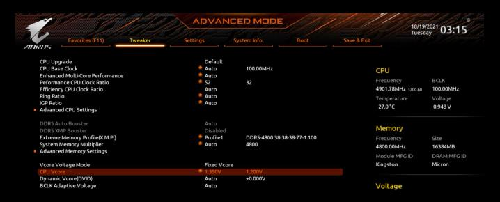
**CPU Vcore**: Raising this helps keeps the system stable at higher CPU frequencies. However, it also increases the amount of heat your CPU produces. We suggest you keep Vcore under 1.4V depending on your CPU cooling solution. Some CPU's should be able to overclock to 5.1-5.2GHz on all the cores at this voltage, however CPUs are not all created equally. Some may need more voltage, some less.
