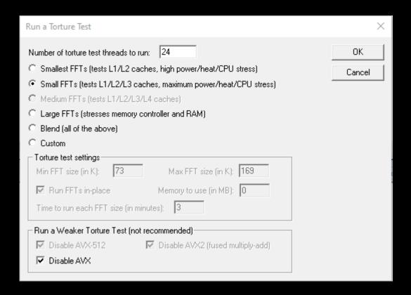
**Step 2:** Start Prime95 and look at "CPU Load" in the Hwinfo64 app. If one of your cores is not at 100%, your system gets the blue screen of death or just freezes, that means your settings were too aggressive and your CPU has failed the stability test. We normally test for 1 hour. You can keep it running overnight for increased assurance.
