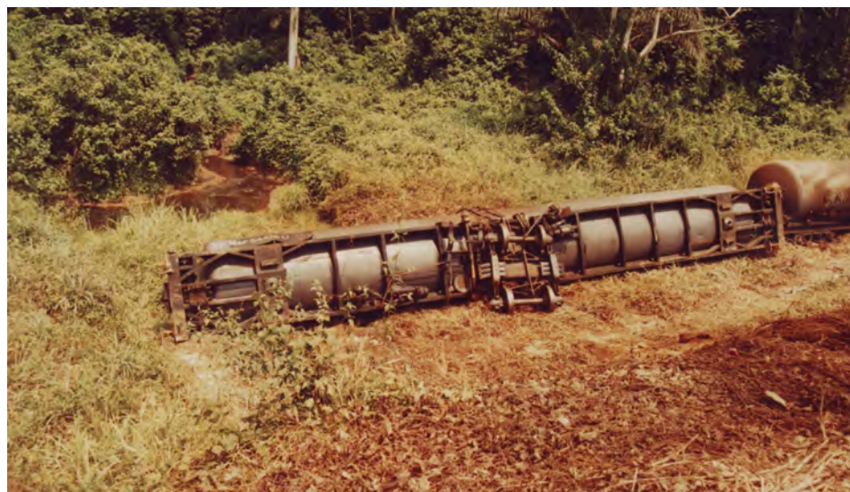
Plate A.2.6: Derailed Camrail wagons next to the Lebby Stream
