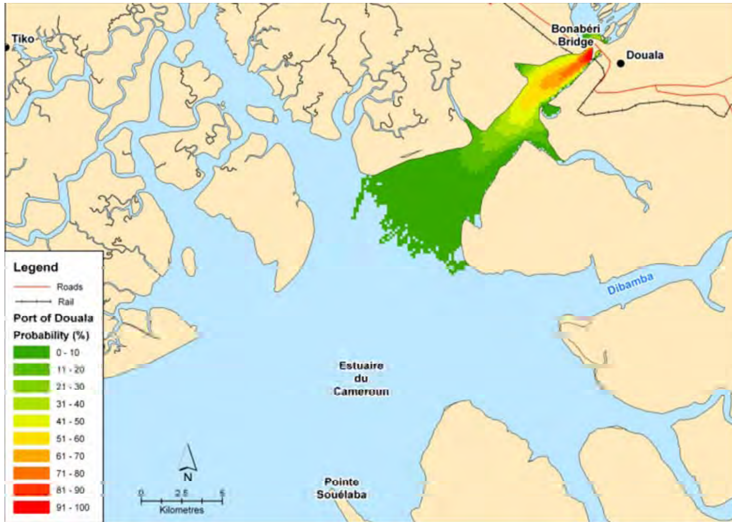
Figure A.2.9 (a): Contour plot showing the predicted probability of exposure to locations from a release of HFO from a vessel berthed within the Port of Douala
