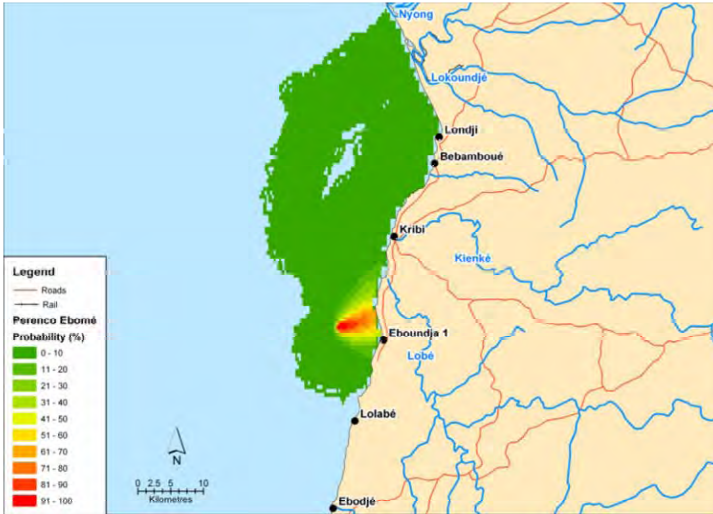
Figure A.2.5: Contour plot showing the predicted probability of exposure to locations from a release of oil from Perenco's Ebome concession.
