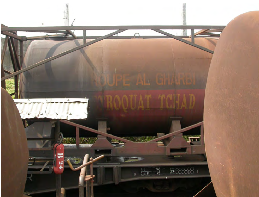
Plate A.2.5: Small rail truck (16 500 l) carrying containerised diesel destined for Chad
