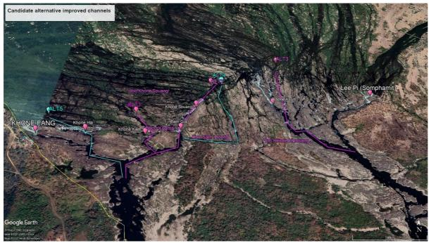
Figure 4-1. Proposed new channels improvements in Khone Fang area
