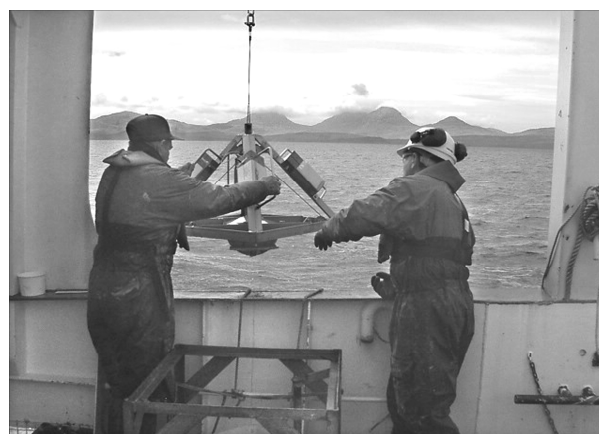
Fig. 1. Deploying the seabed grab sampler in the Sound of Jura.
