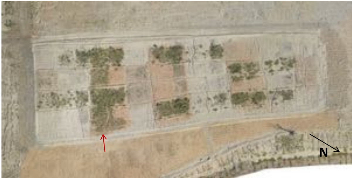
Plate 5.5 Aerial of experimental site taken in June 2014. Refer to Figure 3.1 for position of treatments. The orange coloured subsoil is visible on this aerial, and the OGM treated areas have the highest plant cover as does the mulch treatment on blocks 1 and 4 (red arrow). Treatments are not perfectly contained within their theoretical outlines and contamination of some plots is evident.
