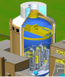
AP1000™ PWR type light water reactor
