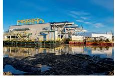
A dewatering 'mega-barge' developed by Weir Minerals Canada
