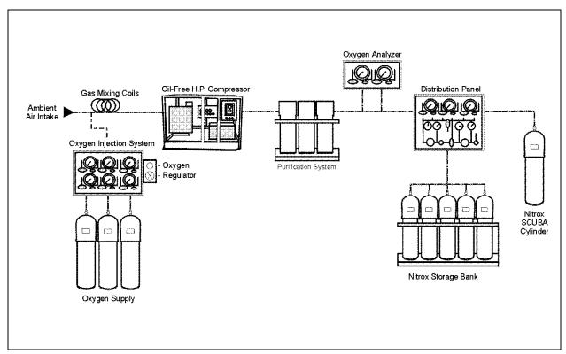
Figure 10-3. Nitrox O<sub>2</sub> Injection System.
