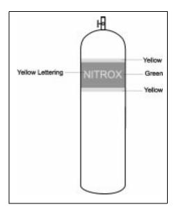
**Figure 10-2.** NITROX Scuba Bottle Markings.
