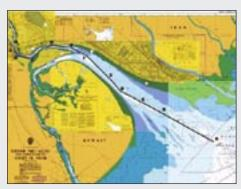
HMS BROCKLESBY led the initial Surface MCM group controlling SWIMS, followed by the command MCMV, USS DEXTROUS plotting and reporting seabed contacts to the rest of the force. The following MCMVs then relocated, detected and destroyed mine-like contacts thereby widening the channel.
