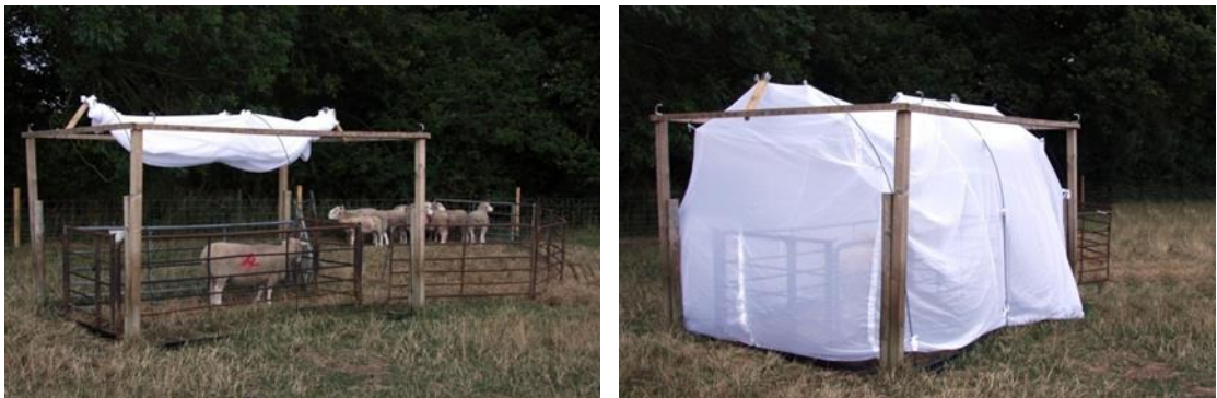
Figure 3.1. Drop trap apparatus used for on-animal collections of Culicoides showing netting up and down
