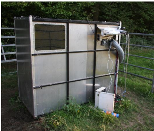
Figure 4.3. Schematic diagram of air flow through air entrainment unit (courtesy James Cook, Rothamsted Research) and the air entrainment unit in situ with ventilation duct attached to an exhaust fan and the delivery of odours to the unlit suction-trap
