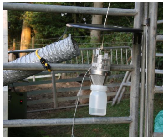
Figure 4.3. Schematic diagram of air flow through air entrainment unit (courtesy James Cook, Rothamsted Research) and the air entrainment unit in situ with ventilation duct attached to an exhaust fan and the delivery of odours to the unlit suction-trap
