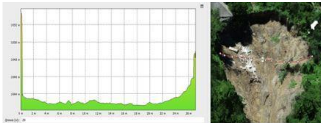
Fig. 6: Transverse profile of the landslide detachment niche
