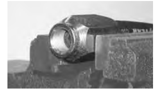
Visually check hose position inside socket.
