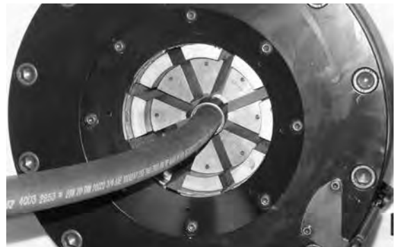
Insert hose assembly into crimper die set.
