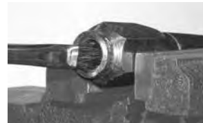
Apply lubricant to stem and hose tube.
