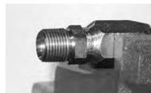
Stem properly seated against socket.
