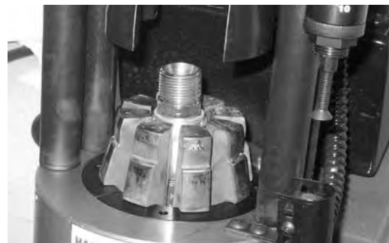
Insert hose assembly into crimper die set.
