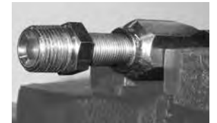
Screw stem into socket.
