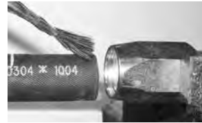
Apply lubricant to hose cover.
