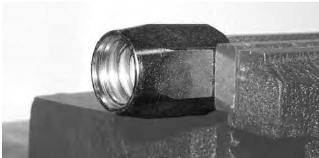
Socket positioned in vice.
