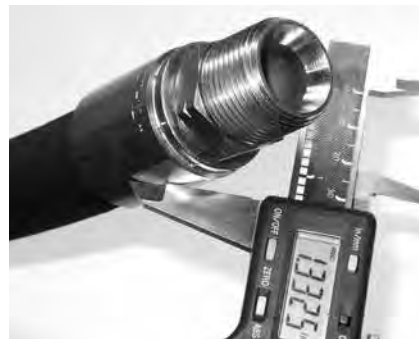
Verify crimp diameter with calipers.
