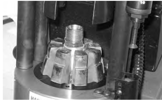
Insert hose assembly into crimper die set.
