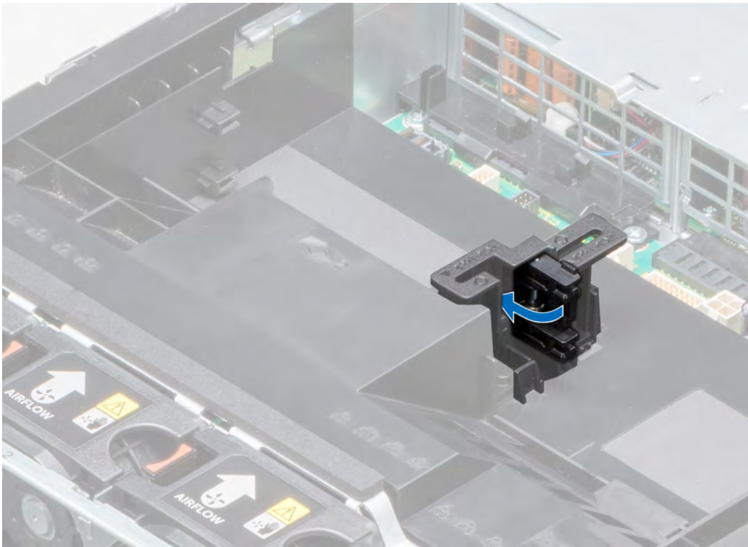
Figure 82. Closing the PCIe card holder latch
