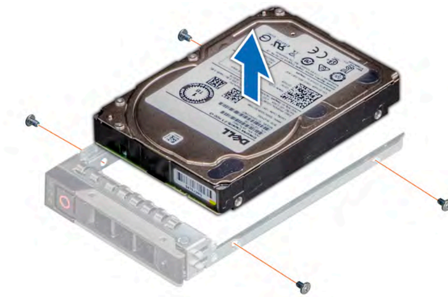
Figure 64. Removing the drive from the drive carrier
