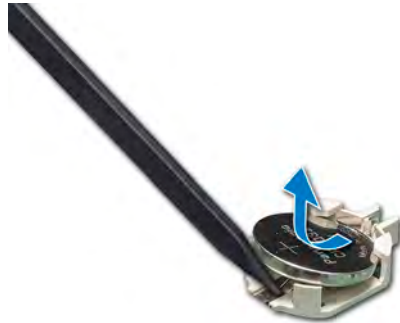
Figure 155. Removing the system battery
