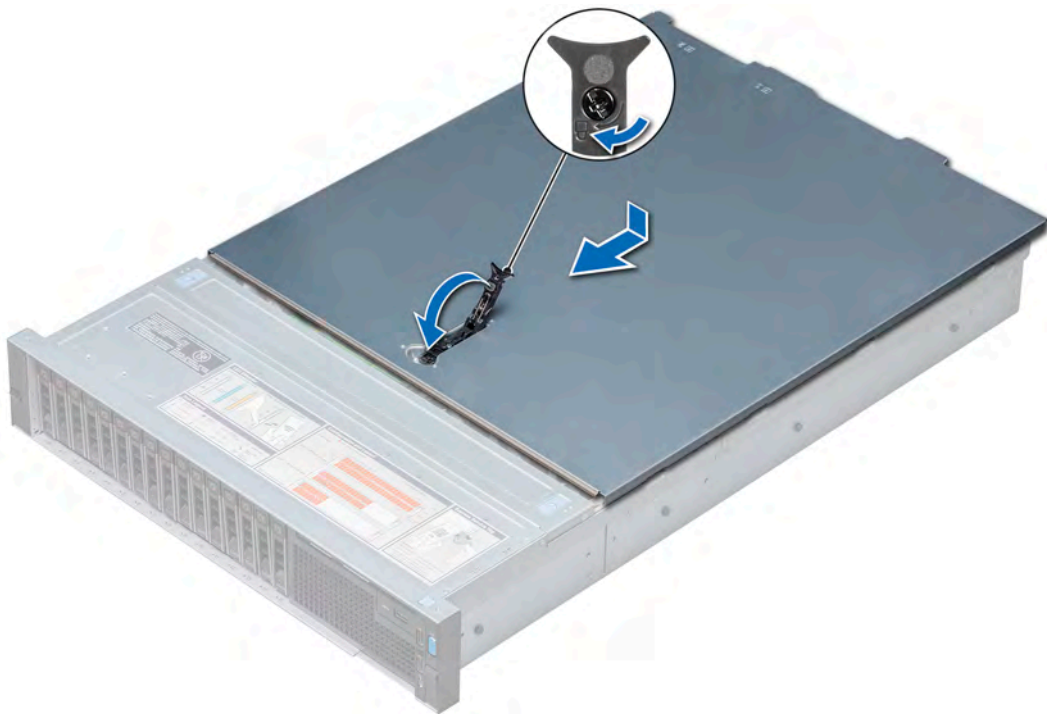
Figure 27. Installing system cover
