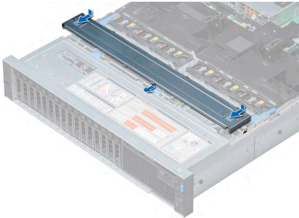
Figure 29. Installing the backplane cover
