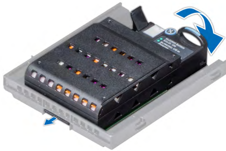
Figure 45. Installing NVDIMM-N battery into the bracket
