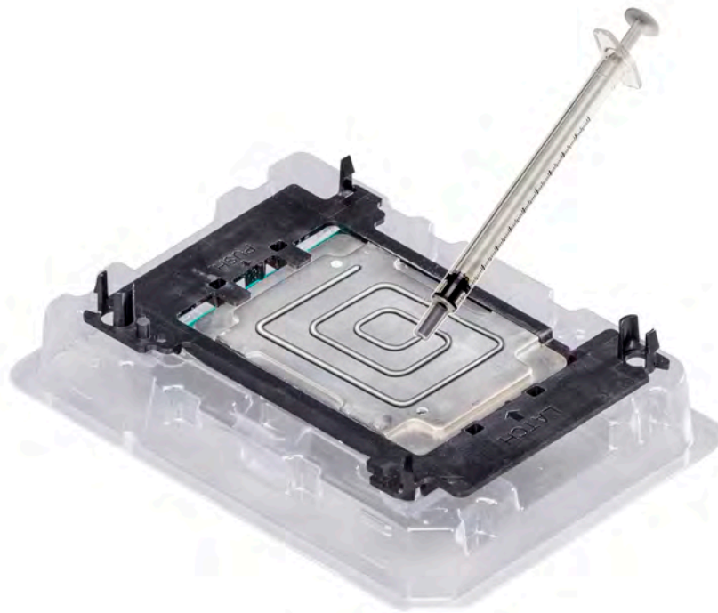
Figure 77. Applying thermal grease on top of the processor
