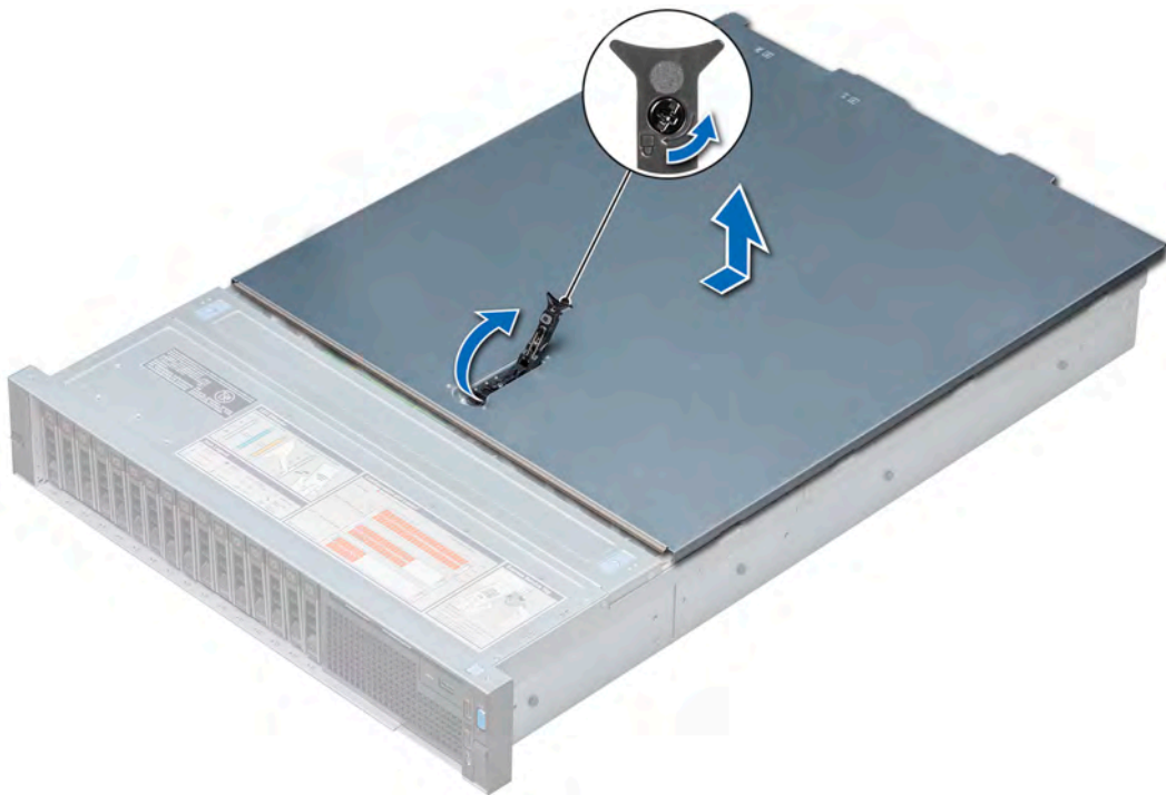
Figure 26. Removing the system cover
