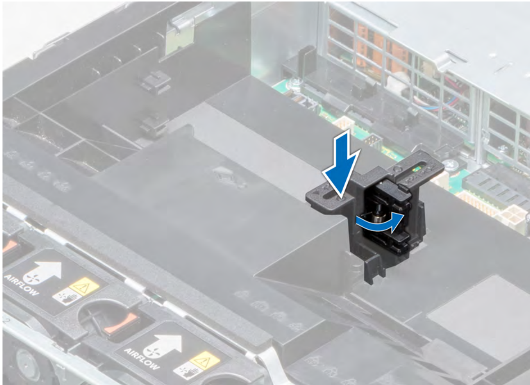
Figure 81. Opening the PCIe card holder latch
