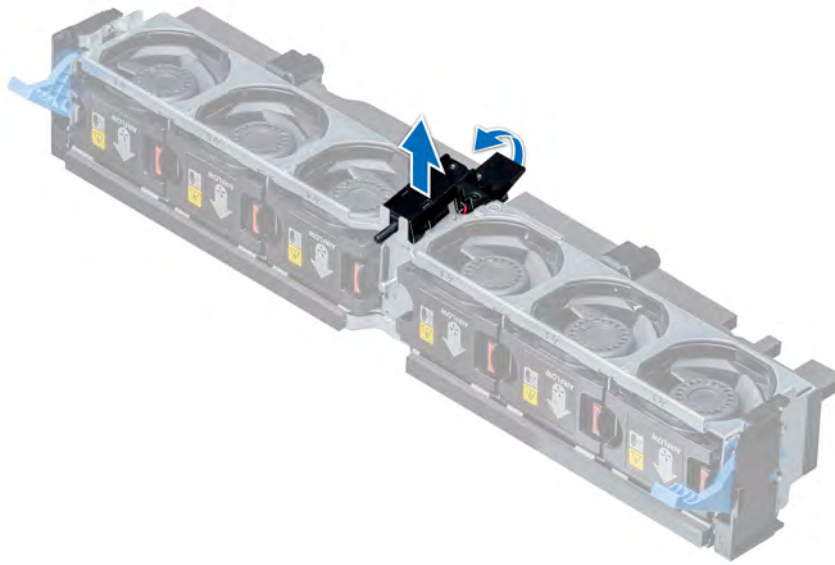
Figure 38. Removing an intrusion switch
