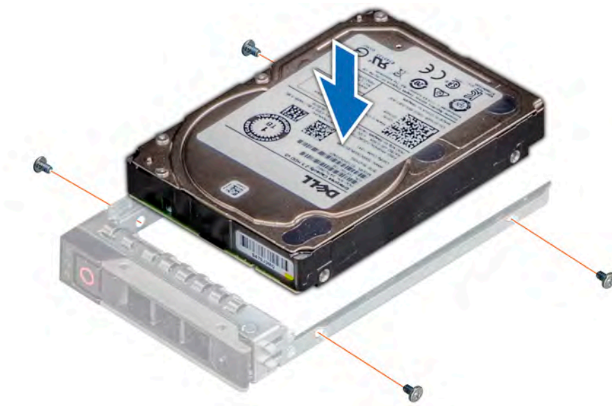
Figure 65. Installing a drive into the drive carrier
