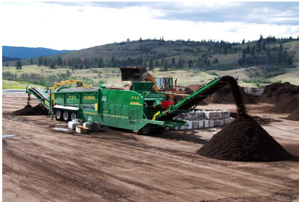
McCloskey 733 RE Trommel in-use (Taken from: https://mccloskeyinternational.com/product/733-re/ )
