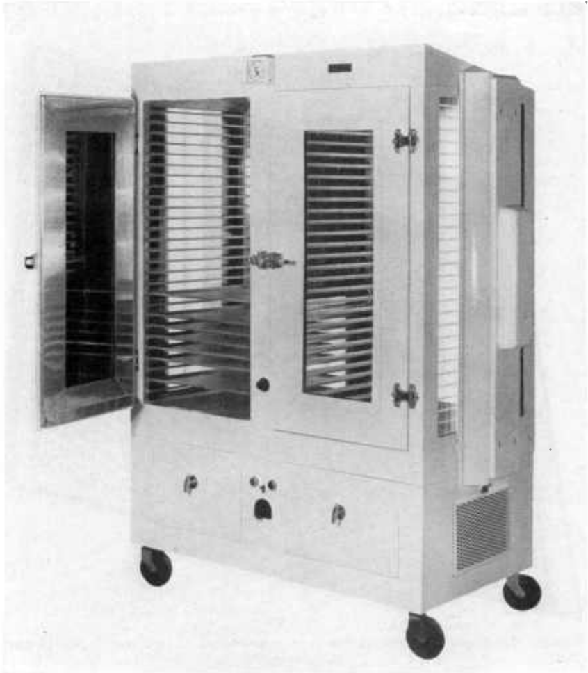
FIGURE 20.—Commercial model daylight germinator. The refrigeration unit is at the bottom of the chamber.
