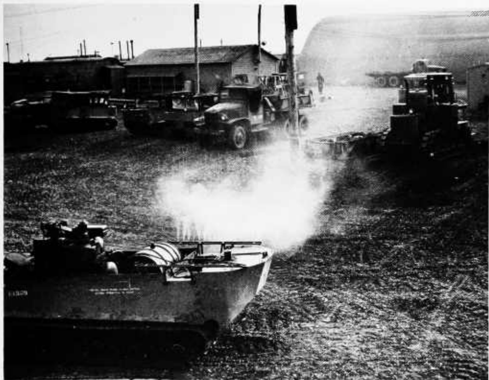
FIGURE 21.—Weasel trailer equipped with compressor and insecticide tank, releasing aerosol for protection of personnel at Umiat. (Photograph by Charles Wilson.)
