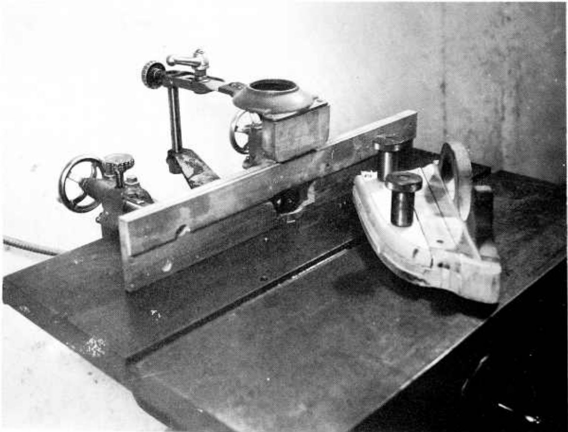
FIGURE 8.—Finished shaping held in the jig used in the test.
