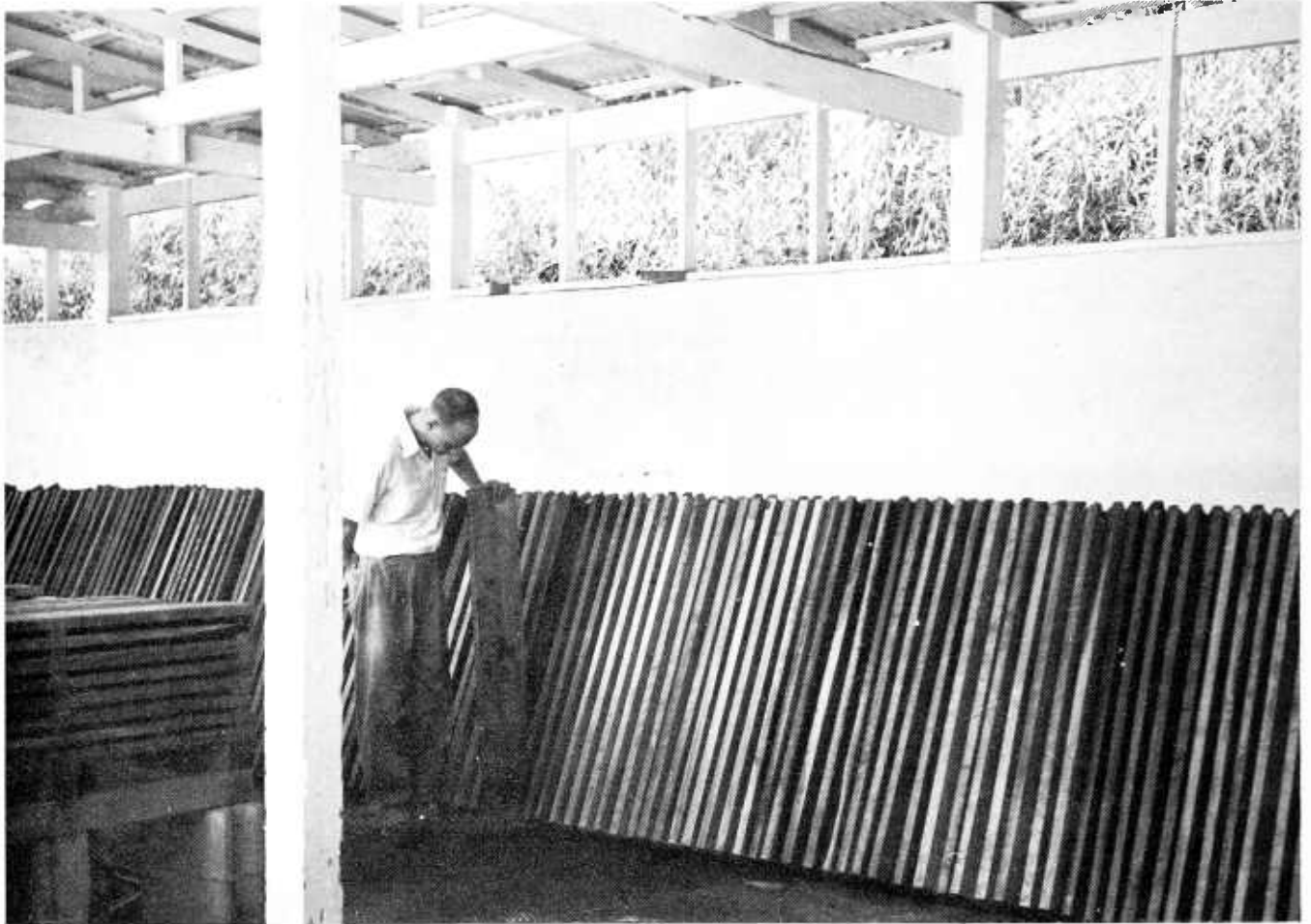
FIGURE 3.—Four-foot boards end-racked for drying, a test of tendency to warp.
