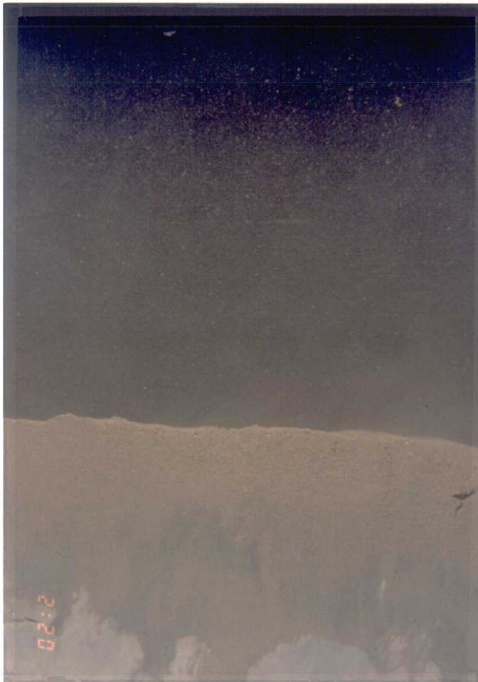
Figure 5-3. Sediment profile images: clayey sediments from a) Station 26 replicate A, with a clearly defined clay layer (lighter-colored sediment) beginning at 6 to 8 cm below the surface; and b) Station SA10 replicate A, with light-colored spots of clay in the lower portions of the image. Scale = 0.65 \times actual size.
