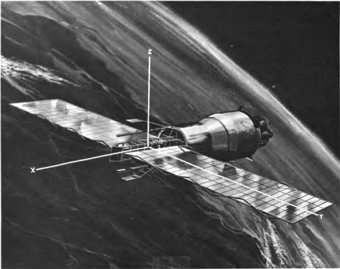
Pegasus satellite configuration with body-fixed coordinate axes indicated.
