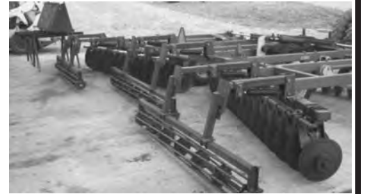
25' Krause 4900 fitted with rolling harrow.
