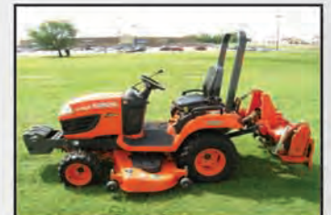
2009 Kubota BX2660 Package, 25hp, 56 hours, 4WD, hydrostat, 60" mower, 48" Bush Hog Tiller and 48" Bush Hog Cutter.....$11,900
