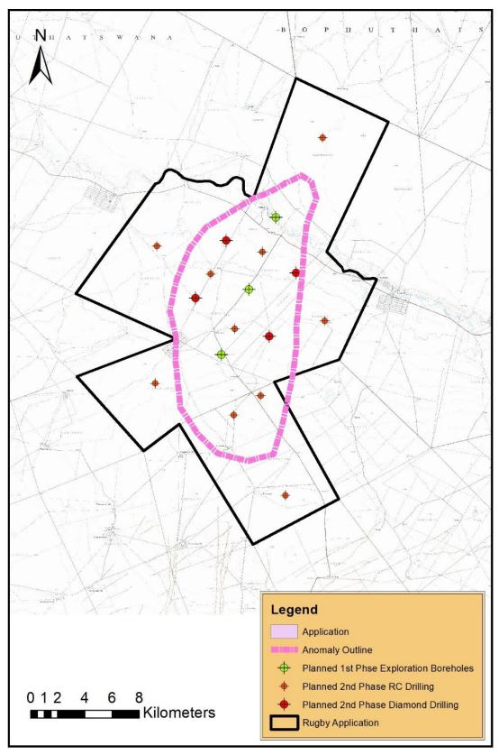
Figure 2: Proposed Exploration Boreholes
