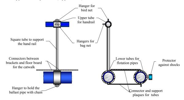
Figure 13: Brackets to hold the flotation and handrail pipes forming the structure of the cage and supporting the floorboards of the catwalk.
