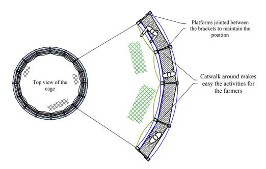
Figure 14: The catwalk around the cage will hold the brackets in its place and will facilitate feeding and maintenance.
