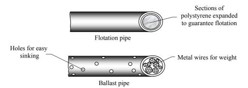
Figure 12: Details of the proposed flotation and ballast pipes made of high-density polyethylene (HDPE).
