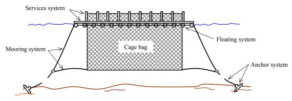
Figure 6: Principal components of the cage for farming.
