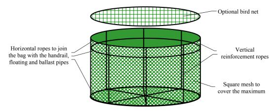
Figure 15: Cylinder cage bag with vertical and horizontal ropes for reinforcement and joints with the rings.
