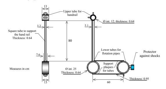
Figure 18: Parts and measures of the bracket.
