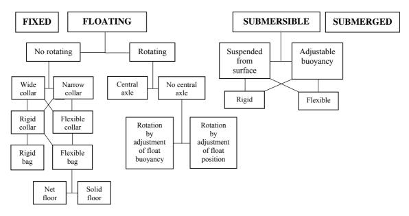
Figure 1: A classification system for cages by way of operating (Beveridge 1996).
