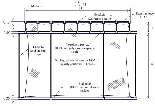
Figure 17: General arrangement of parts of the cage.
