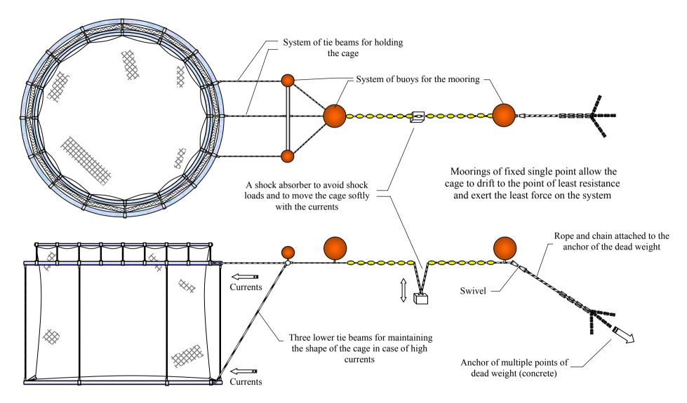
Figure 16: Moorings and anchor systems proposed for the cage for farming Black Snook in Santa María La Reforma Bay, Gulf of California.
