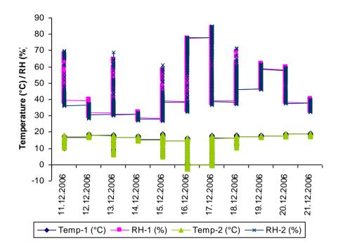
Figure 14: Temperature and humidity (RH) profiles during the drying process (logger 1 and 2 in front of and behind the drying racks).
