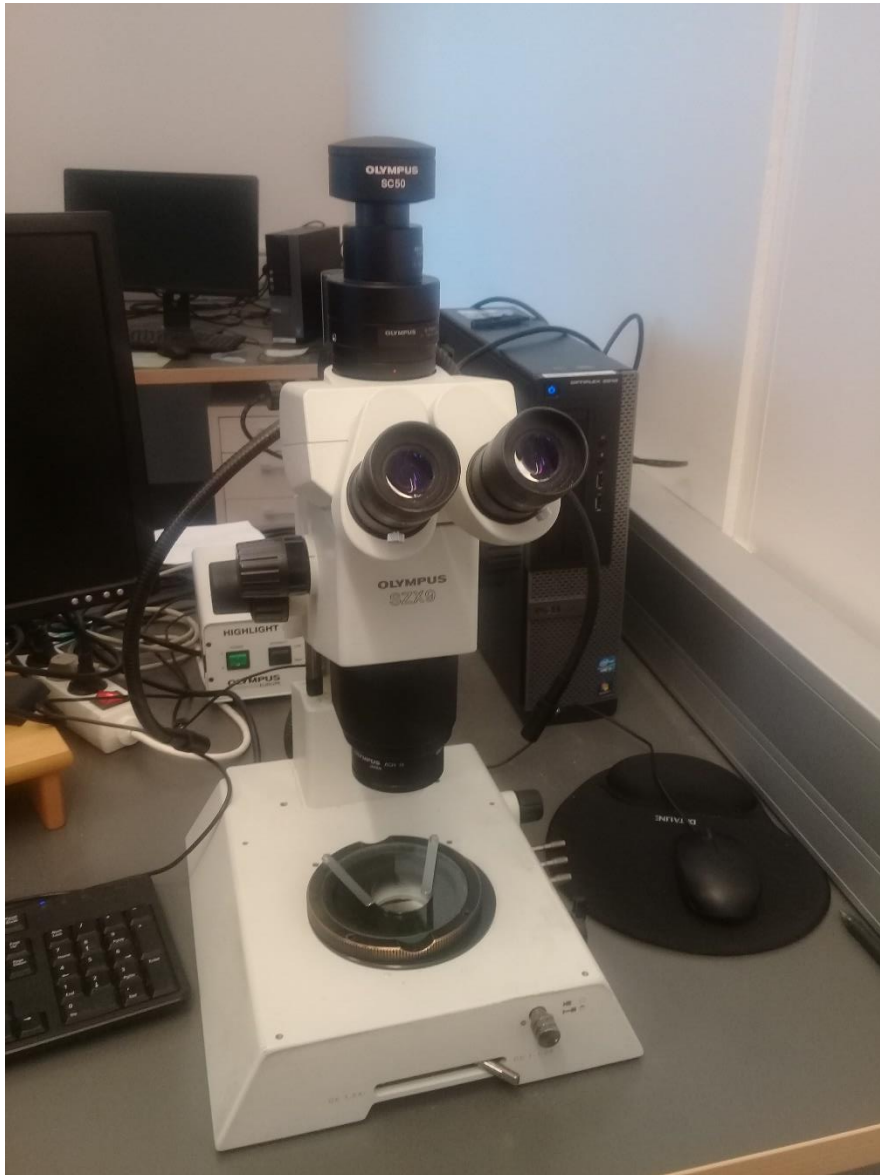
Stereoscope Olympus SZX9 connected to a camera Olympus SC50, they were connected to a screen monitor.
