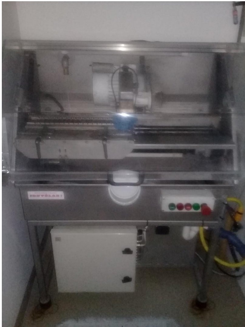
The otolith cutting machine used in the process.
