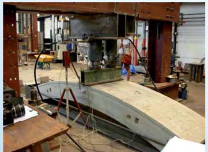
Dual layer segment during one of the project tests.
