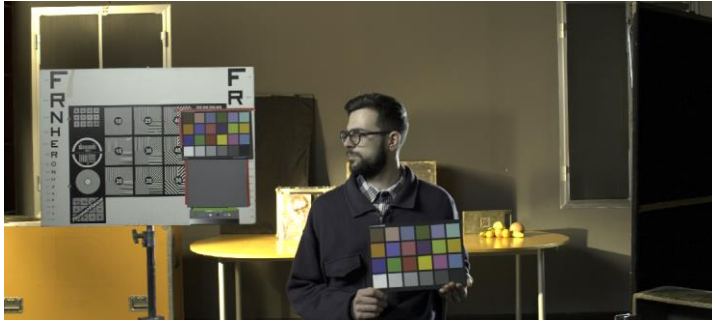
Fig. 4 – Footage from Fig.3's set (Sony F55 camera), after applying the Input Transform and an LMT into ACEScsc colour space for the purpose of colour grading (washed out look is due to the tone-curve behaviour of the RRT).
