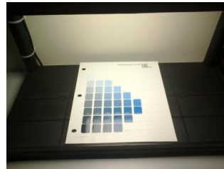
Fig. 3 – Viewing booth with standardised lighting of Munsell charts.
