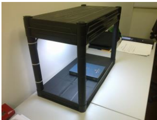
Fig. 3 – Viewing booth with standardised lighting of Munsell charts.
