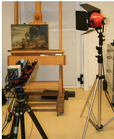
Fig. 1 Picture of the set during a hyperspectral video acquisition.
