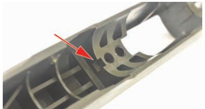
Above: In the Winchester, a steel recoil lug (top arrow) has been inserted into the polymer stock and mates nicely with a mortise (bottom arrow) on the bottom of the action, just in front of the forward action screw.
