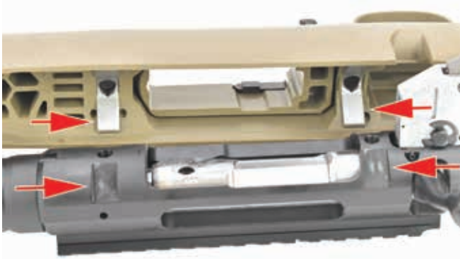
Above: The Ruger's bedding blocks are steel V-shaped inserts (top arrows) designed to draw the action tightly to the stock and aid accuracy. The stock blocks fit into corresponding slots in the action (bottom arrows).
