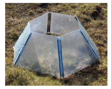
Passive open-top fiberglass chambers Increase temperature 1-3° C
