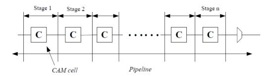
Figure 1.9. A unit split pipelining.
