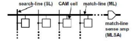
Figure 1.2. The basic circuit configuration of a CAM word
