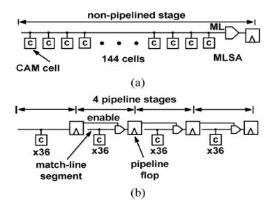
Figure 1.7. (A) Non-pipeline stage, (ii) pipeline stage is divided into four segments.
