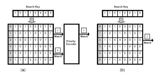
Figure 1.3. T-CAM with (a) Global masking, and (b) local shelter.
