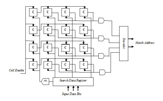
Figure 4.2. Parity based PBCAM architecture.
