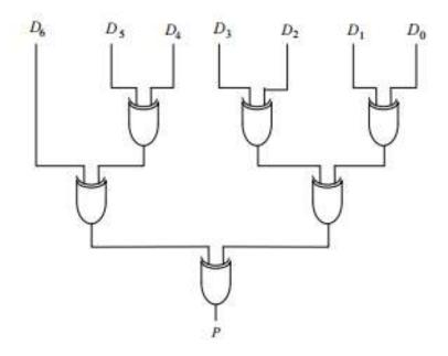
Figure 4.1. The parity parameter extraction logic circuits.
