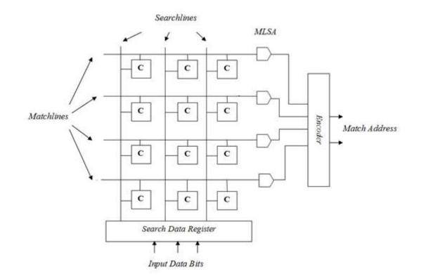
Figure 3-1. Conventional CAM architecture.
