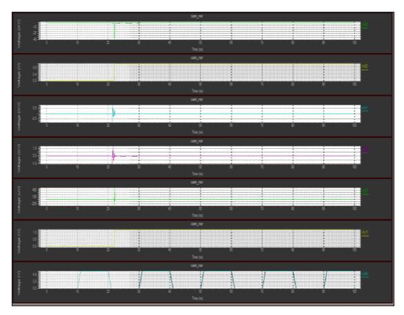
Figure 5.2. Simulation Waveform of Conventional CAM Design in W-Edit.
