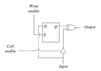
Figure 1.1. CAM cell circuit unit [1]
