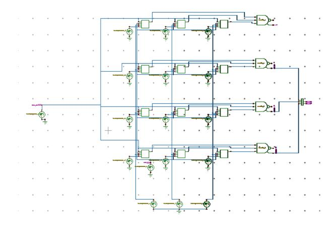
Figure 5.1. Schematic of Conventional CAM in S-Edit.
