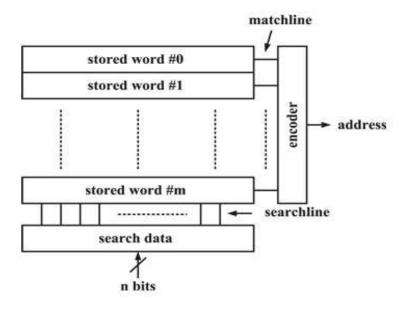
Figure 1.5. CAM conceptual diagram.
