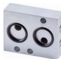
ZPNX 16 Plate to swap the working ports of a NAMUR-valve. Can be used in case pressure- and exhaust ports face into the wrong direction.
