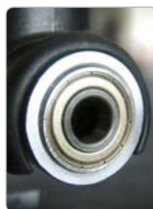
Swivel joint with 2 roller bearings.
