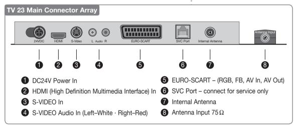
The antenna should be connected to the TileVision® using the Antenna Input (⑧) and not to the Internal Antenna connection (⑦). This allows a Sky<sup>™</sup> or Sky+<sup>™</sup> remote control to be used to change channel on the Sky<sup>™</sup> digital receiver via the infrared sensor in the TileVision®. See page 7 for more information.
