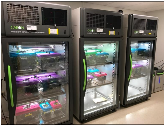
Fig. 2. Chambers that control relative humidity, temperature and light are used to rear snails in the SEPP captive rearing lab.
