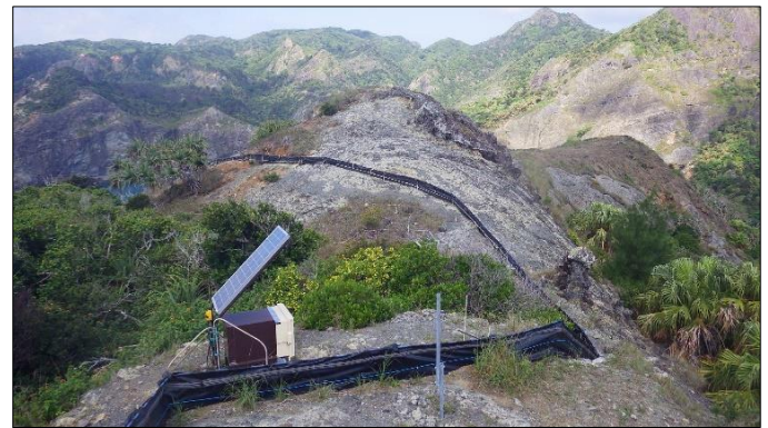
Fig. 2. The electric fences constructed at Toriyama to prevent the spread of P. manokwari .
