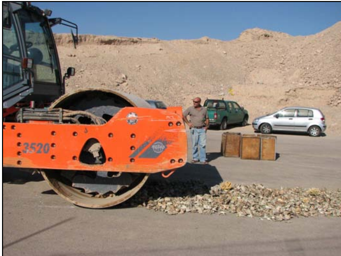
Fig. 2. Road-roller ready for crushing the shells and corals. In the background some of the tea-boxes.
