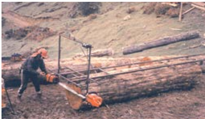
Flitching on site - rimu ( Dacrydium cupressinum ), with an 'Alaskan' technique. Source: Simon Stokes
