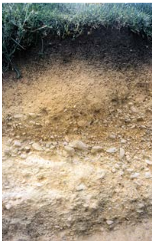
A version of the Poporangi soil found throughout mid-Hawke's Bay, with gravels deposited over loess giving a false impression of a soil with good drainage ability, when, in fact, water will perch. Source: Simon Stokes
