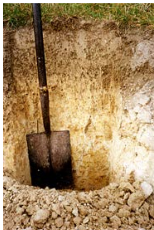
Matapiro soil, shallow ash with loess and duripan at 50cm. Source: Simon Stokes
