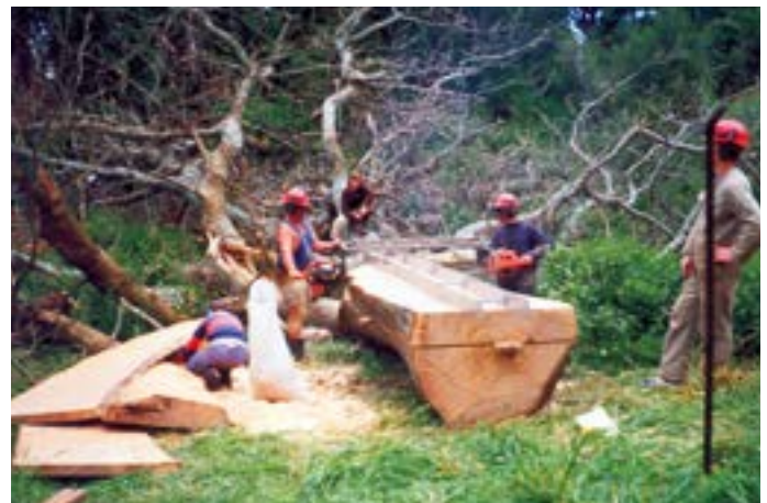
Milling an old oak on-site on the Mackintosh property, Matahorua Road, Putorino. Source: Susan Mackintosh
