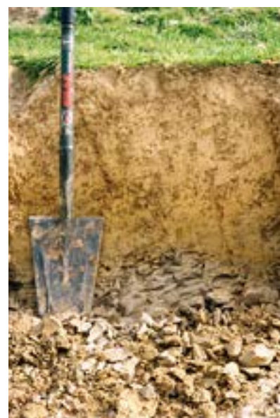
Recent steepland soil development on mudstone near Atua Road, Elsthorpe. Soil developing on an old eroded site. Note the lack of topsoil. Source: Simon Stokes
