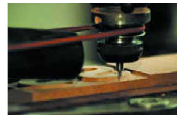
Using the pantographic articulated joint system of the wooden type mill (middle photo) Janssen transfers a letter template in miniaturized form onto the wood block (photo below).
