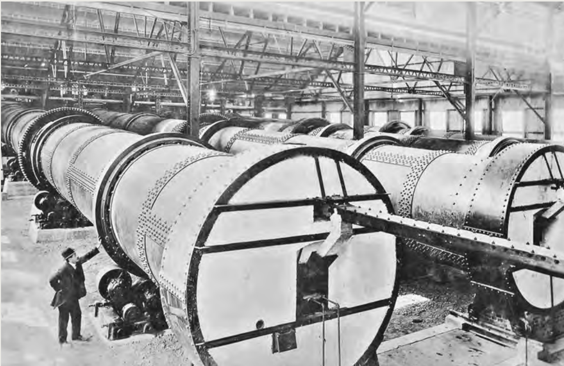
Charles A. Matcham (*15/01/1862 Torquay †22/09/1911 Allentown), founder of the Lehigh Portland Cement Company by the rotary kilns in Evansville, 40 km south-west of Allentown, Pennsylvania, shortly before commissioning, 1909
