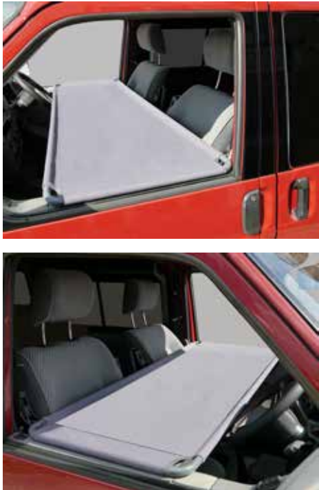
Collapsible 'tent pole' frame construction – rests on door tops and held in place by seats and dash board.
