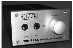
The OBH-21 is a miniature audio amplifier specifically designed to drive two pairs of low to medium impedance  $(30\Omega$  -  $300\Omega)$  headphones from a line level source.
