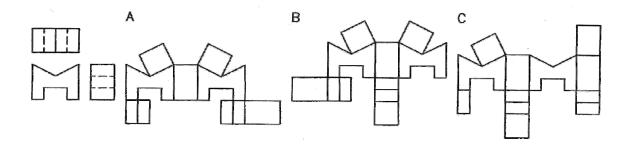
\_\_\_\_\_3. The rectangular prisms shown in isometric below have markings on each of their four long sides. Choose the panel for the flat pattern so that when folded up, the correct object is obtained.
