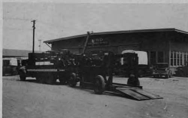
DESIGNED TO REDUCE shipping problems at the busy Navy Yard, the mobile grease rack for finger lifts shown above was constructed by Chief Petty Officers, C. E. Colvin and Perry Brown.
