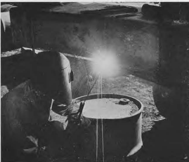
Arc welder at work repairing rooster.
