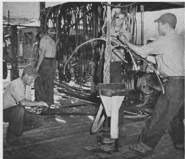
Splicing wire rope in bosun's locker.
