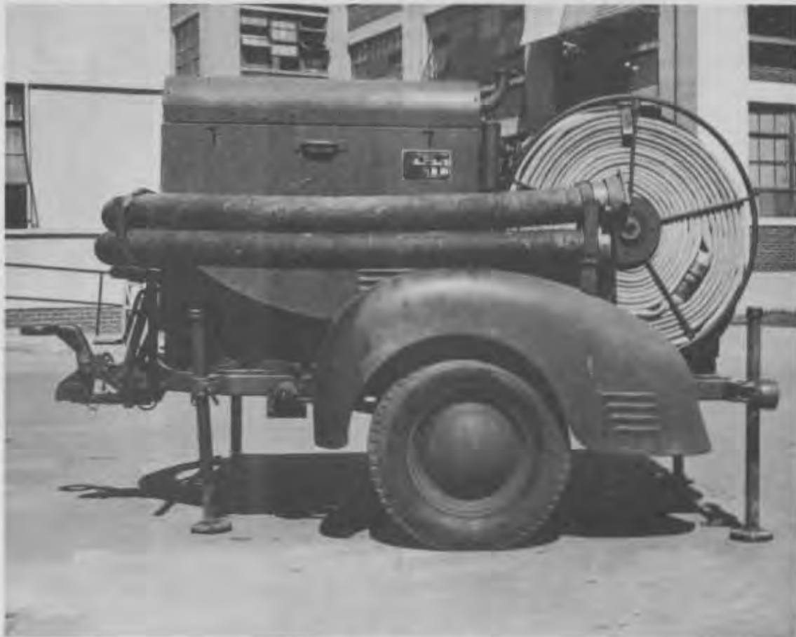
TRAILER FIRE PUMP (2H93)
