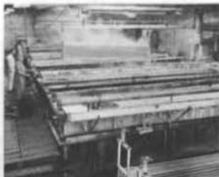
Anodizing tanks. A load of extrusions are being moved to the next tank. This electrolytic process seal the surface of the metal against corrosive salt water.
