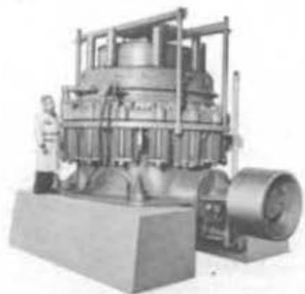
7-foot Short Head Symons Cone Crusher with hydraulic clamping and adjustment.
