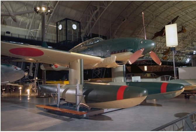
Aichi M6A1 Seiran at the Udvar-Hazy Center. Aichi chief engineer Toshio Ozaki designed the Seiran (Clear Sky Storm) during World War II to fulfill a requirement for a bomber that could operate exclusively from a submarine. (Photo from Udvar-Hazy Center; Smithsonian web ID: WEB10862-2008)
