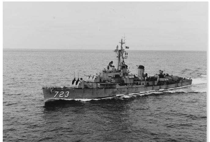
USS Walke (DD-723) underway in East Asian waters, 23 November 1953. Note that Walke has been refitted with 3-inch/50-caliber guns by this time, replacing her original 40mm battery (NH 99810).
