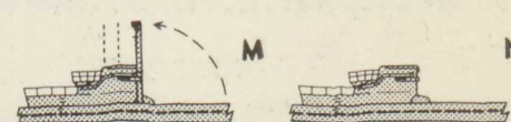
VII. Folding snorkel of ex-German "TYPE IX-C" CLASS. Shown in upright position in M and secured in a slot out into the deck in N.
