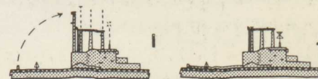
V. Folding snorkel of British "A" CLASS. Shown in upright or operating position in I and secured in J.
