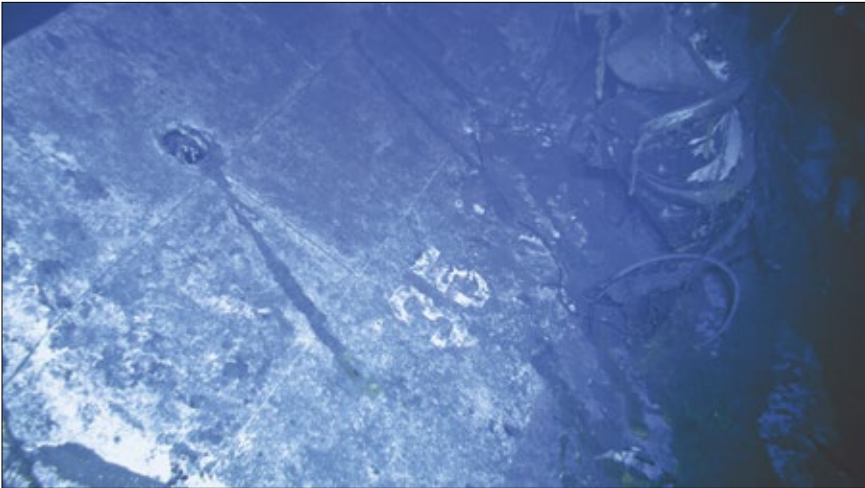
Figure P-2. An image taken by a remotely operated vehicle shows what appears to be the painted hull number “35.” Based on the curvature of the hull section, this seems to be the port side of the ship. Using Figure 2-1 as a reference (see page 45), the number is painted in the same font, and the “3” aligns with the circular feature above it in both photos. Photo courtesy of Paul G. Allen
