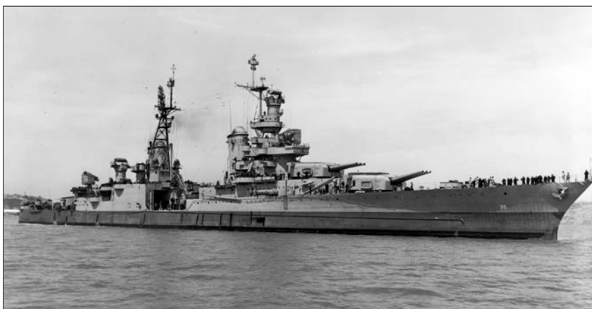
Figure 2-1. View of starboard side of Indianapolis (CA-35) off the Mare Island Navy Yard, California, 10 July 1945, after her final overhaul and repair of combat damage. On the night of 30 July two torpedoes fired from Japanese submarine I-58 slammed into this side of Indianapolis at frame 7 (slightly aft of the hull number) and frame 50 (directly below the navigation bridge).
