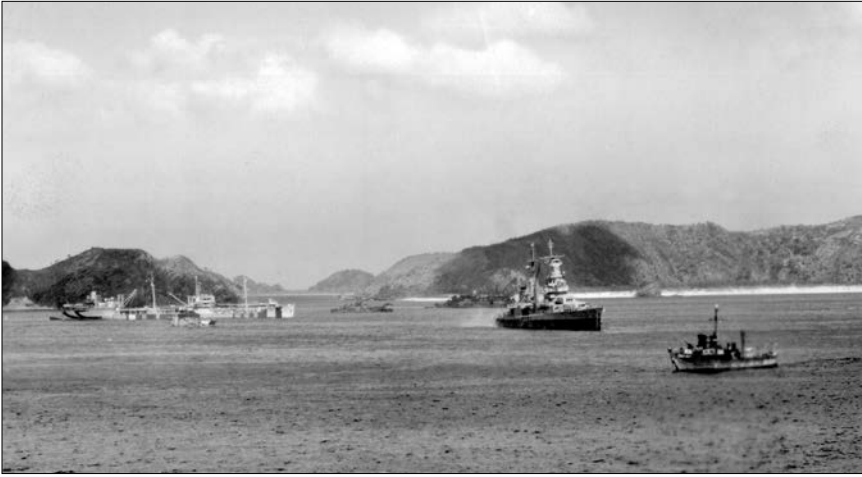
Figure 1-3. The damaged Indianapolis (CA-35) at Kerama Retto, Ryuku Islands, photograph dated 2 April 1945. Indianapolis is listing noticeably and water is being pumped from starboard aft. According to the Indianapolis 's deck logs, from 0300–0600 on 2 April the ship fired more than 300 rounds from its 20mm and 40mm guns at enemy aircraft operating in the area. At 0800, burial services were held for the final two crewman recovered from flooded compartments below deck. At 0855, shortly after the morning burial services, a kamikaze splashed into the water approximately 5,000 yards from a CVE. The photo was taken from New Mexico (BB-40) and YMS-327 is forward of Indianapolis . LCT-1414 is approaching Indianapolis starboard to replenish her spent ammunition. Indianapolis is anchored for repairs prior to her return to Mare Island, San Francisco, for her final overhaul. She arrived at Kerama Retto under her own power on 31 March at 1221, escorted by Twiggs (DD-591). Clamp (ARS-33) moored alongside Indianapolis to port after arriving to assist with repairs.
