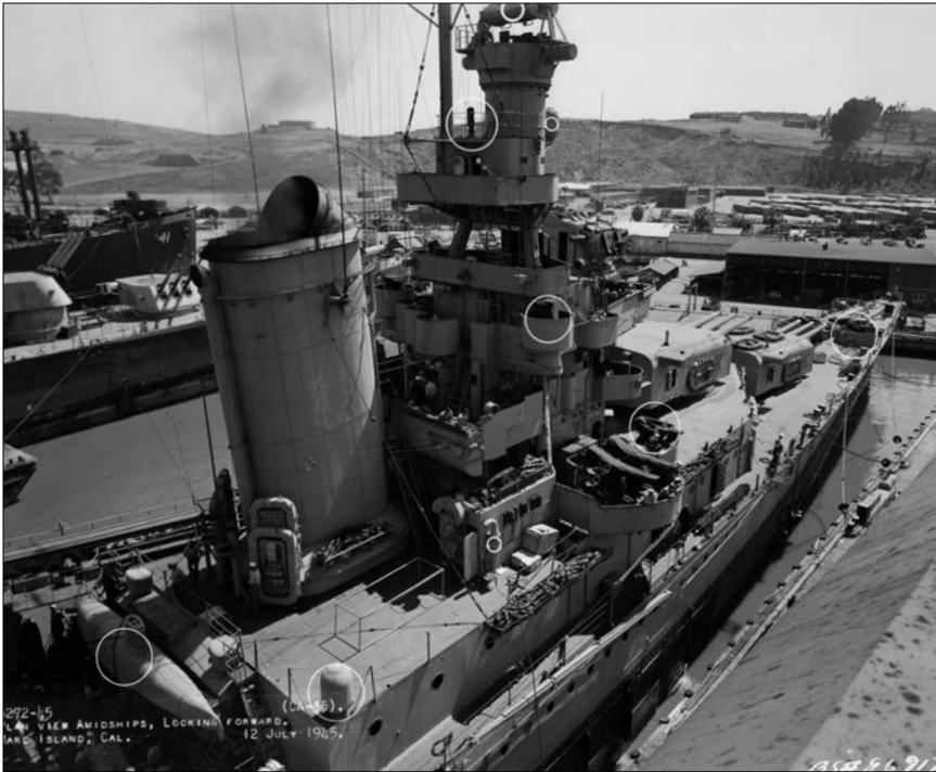
Figure 2-2. Detail view of ship’s forward stack, superstructure and hull, from alongside her starboard side amidships, at the Mare Island Navy Yard following her final overhaul, 12 July 1945—the day that Captain McVay received notification of his top secret mission. Circles on photograph mark recent alterations to the ship. Note the life rafts and floater nets. The ship sunk by the starboard side and went down within 15 minutes of being hit. Many of the life rafts did not release when underwater. Also note the bow of Hercules (AK-41) in the left distance.
