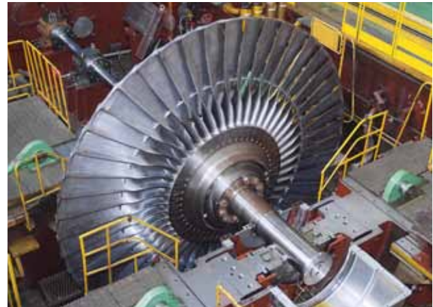
Fig. 13—Rotational Vibration Test. Rotational vibration tests in a vacuum chamber were used to confirm that resonance is avoided.
