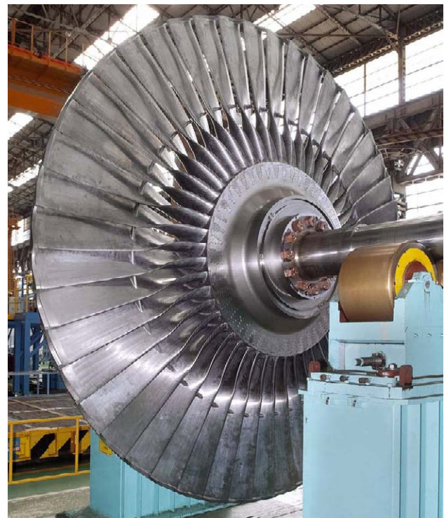
Fig. 1—3,600 r/min 50-inch Last-stage Buckets. With an annulus area among the largest in the world *2 , turbine efficiency is improved by reducing wasted kinetic energy.
