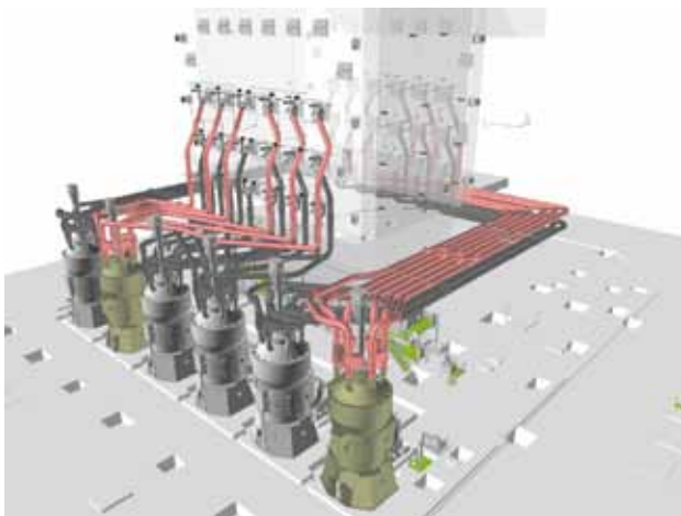
Fig. 6—Biomass Co-firing Facilities Utilizing Preexisting Combustion System.
